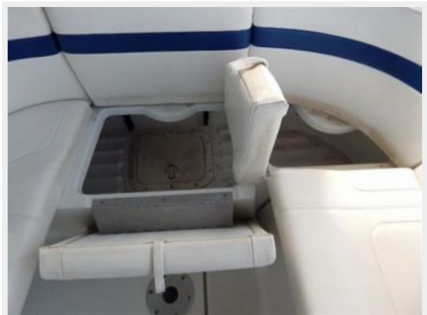
Cockpit Storage Under Settee
