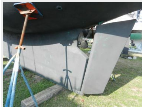
protected prop and skeg hung rudder
