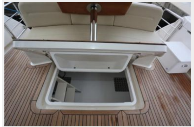
Large Lazarete Entrance Hatch
