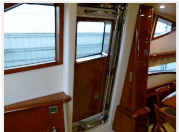
Watertight Door (Starboard Side)
