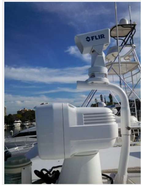
FLIR Infrared & RCL 600 Searchlight
