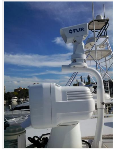
FLIR Infrared & RCL 600 Searchlight
