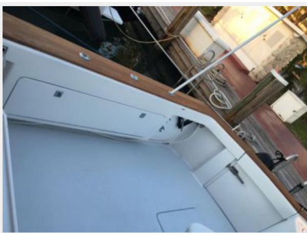
New teak covering boards 2
