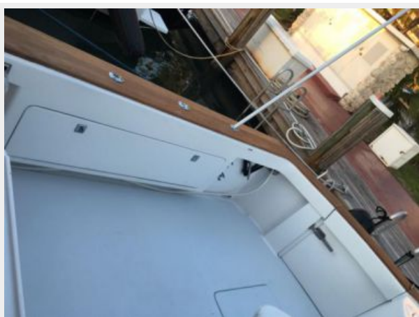
New teak covering boards 2
