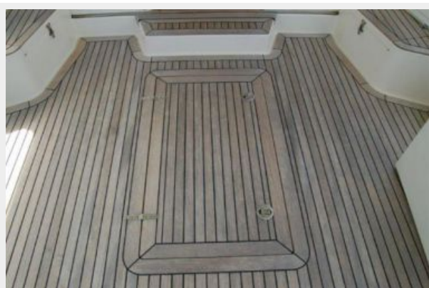
Cockpit Bilge Access
