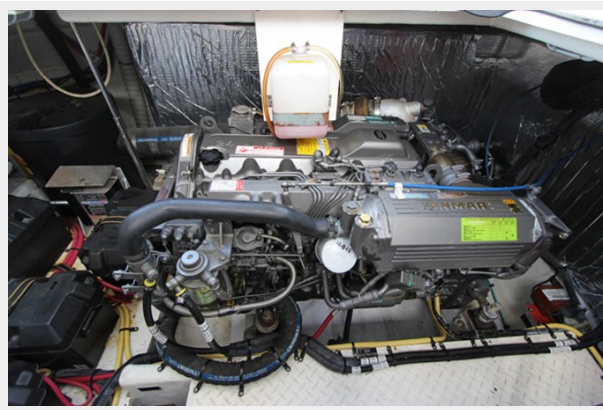
Port Yanmar 6LPA-STP (315HP) Engine w/294 hrs
