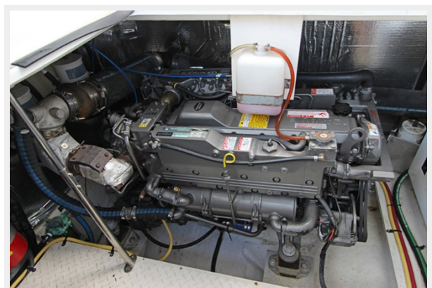
Starboard Yanmar 6LPA-STP (315HP) Engine w/296 hrs
