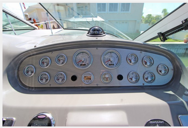
Faria gauges at Helm
