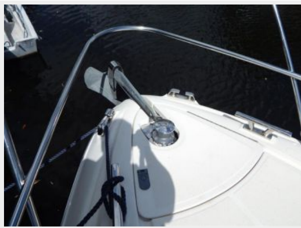
Anchor and Windlass
