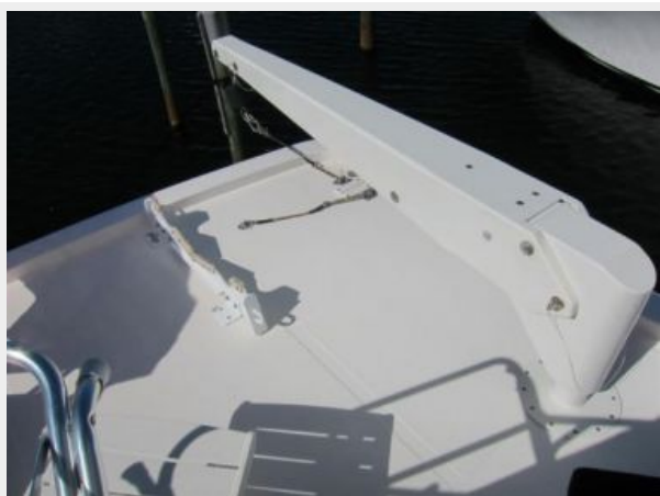
Davit on Upper Deck
