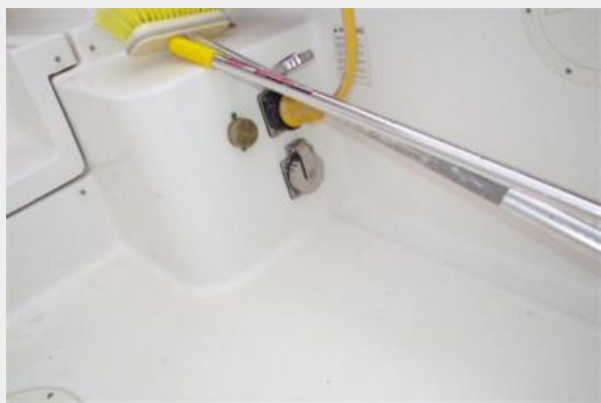
Dockside Power Hook Up
