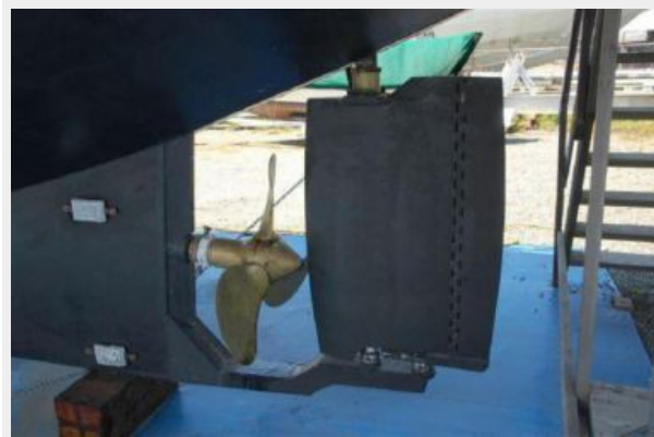
Hundested propellor and articulating rudder
