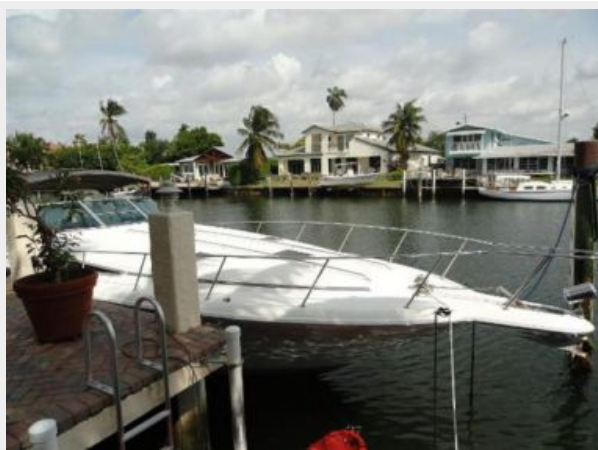
Bow Railing/ Pulpit
