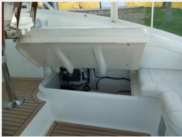
Hydraulic Storage Hatch
