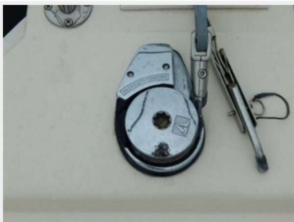
Deck Anchor Windlass
