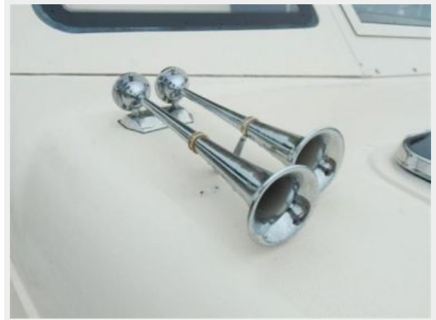
Deck Air horns
