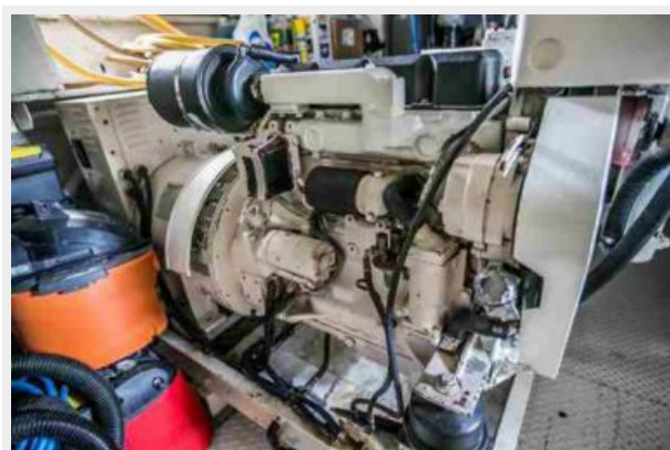
Engine room - 30kw Northern Lights GenSet
