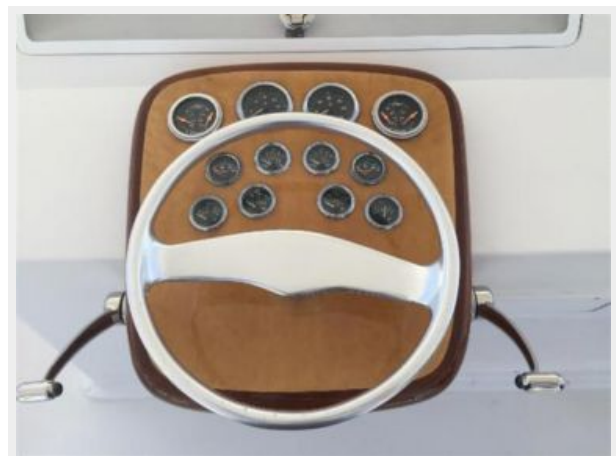
Flybridge - Custom teak helm bubble with single-lever controls, polished stainless steel control handles and steering wheel
