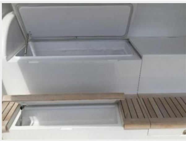
Cockpit Freezer - Freezer & Refrigerator Under Mezzanine
