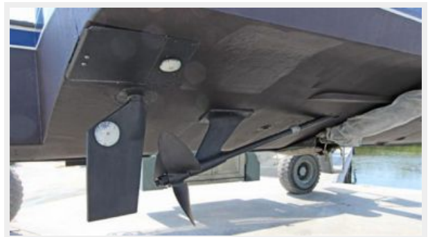
Starboard Rudder & Shaft
