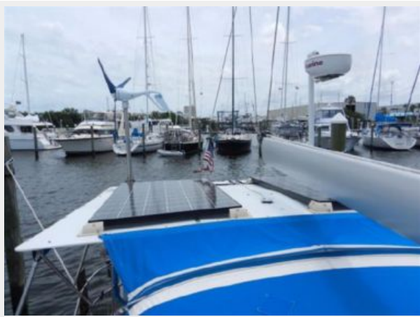
Solar, wind gen and radar
