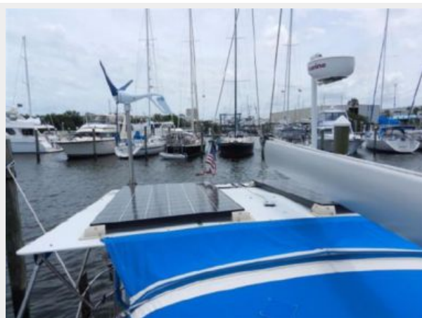
Solar, wind gen and radar
