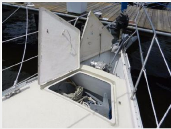
Anchor and windlass lockers
