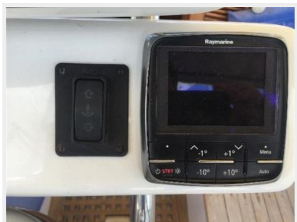
Tayana 42 1979 - Raymarine Linear Drive Unit #2 with X30 Core Pack and P70 Autopilot Control Head – 2012
