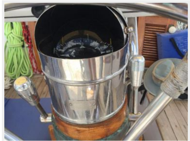
Compass - Ritchie SP5-C Compass rebuilt and a new light (red) installed- 2013
