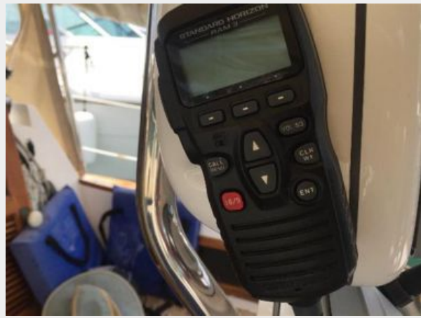
VHF - Standard Horizon GX2150 Matrix AIS VHF with RAM 3 Remote Mic at the Helm – 2013
