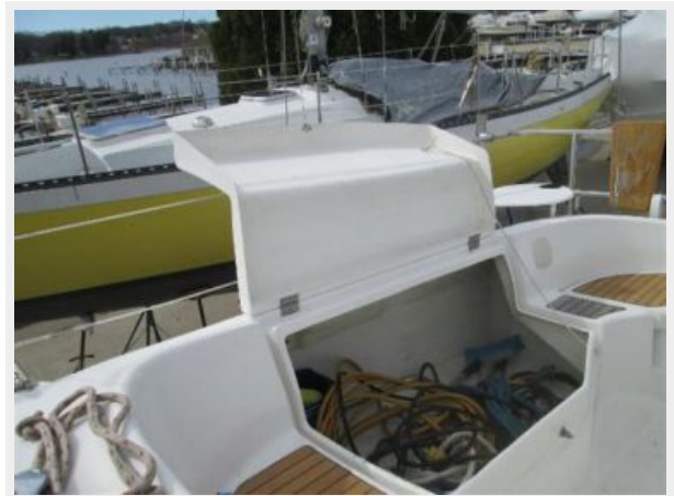
Starboard Lazarette Storage
