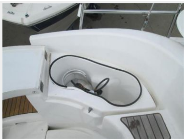
Propane tank storage
