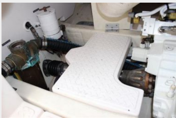
Stbd drive shaft with cover
