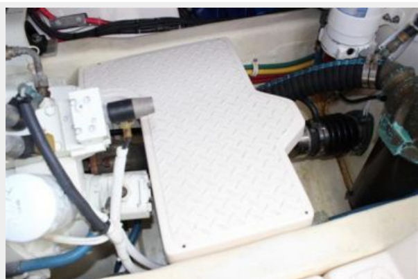
Port side drive shaft with cover
