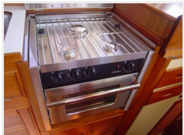
Galley new Force 10 stove
