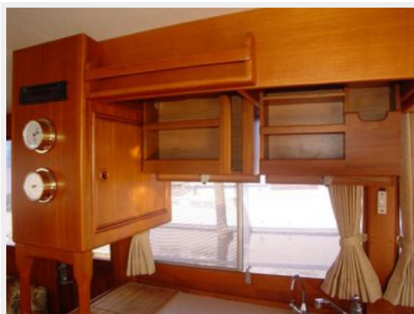
Galley drop down dish lockers
