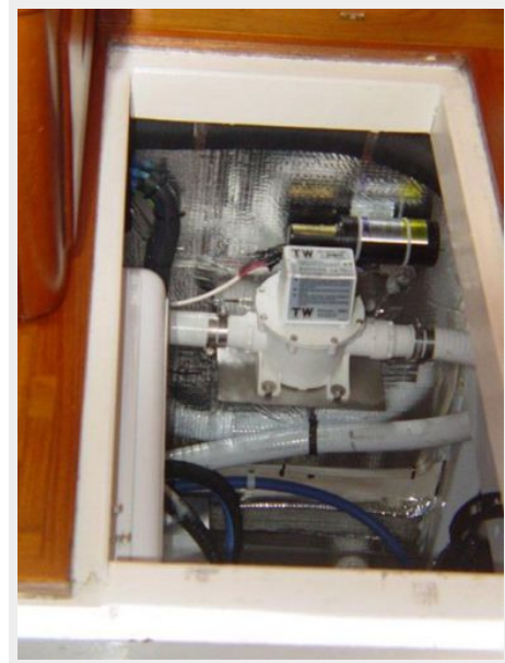
Engine Room VacuFlush system
