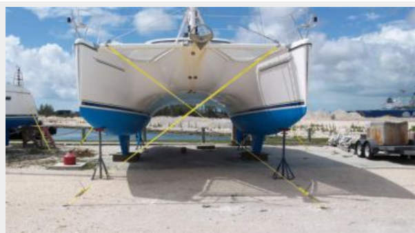
Strapped down for Hurricanes
