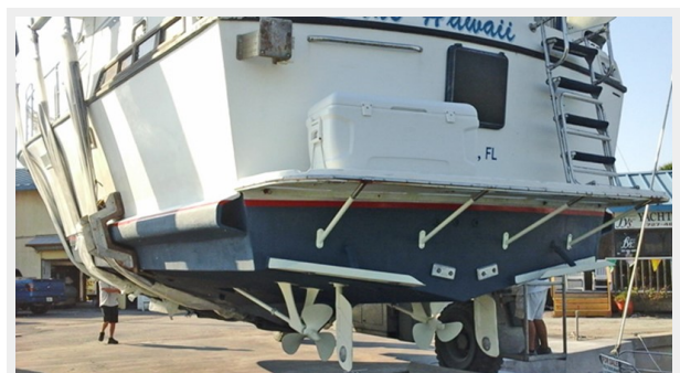
Fresh Bottom Job & New Rudder Glands March 2015
