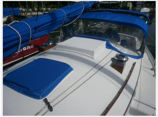
Protective covers over hatch
