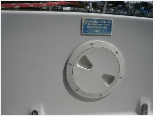
Cover on Emergency Tiller access
