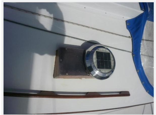
Two Solar Vents Port & Starboard
