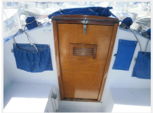
Ventilated Hatchboards w/line & instrument protection
