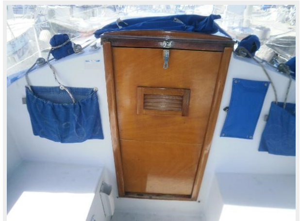
Ventilated Hatchboards w/line & instrument protection
