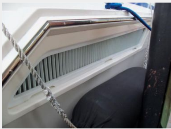
Proper Engine Room Vents
