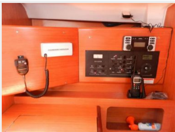
new VHF w/AIS & GPS and electric panel
