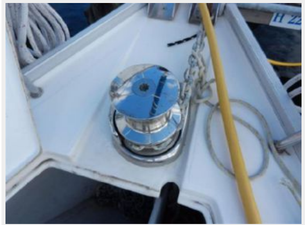
electric windlass w/ handheld control
