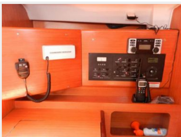
new VHF w/AIS & GPS and electric panel
