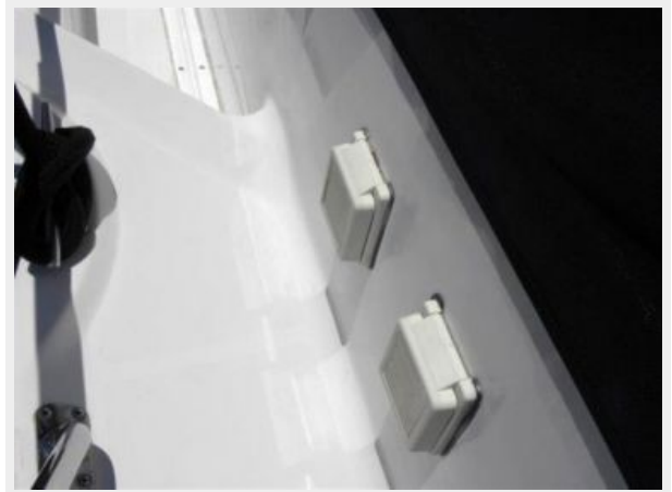
Fordeck shore power starboard side
