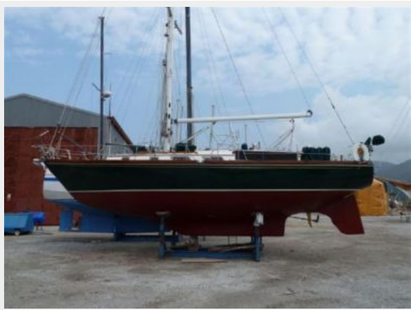
Hull configuration, center cockpit centerboard extended transom
