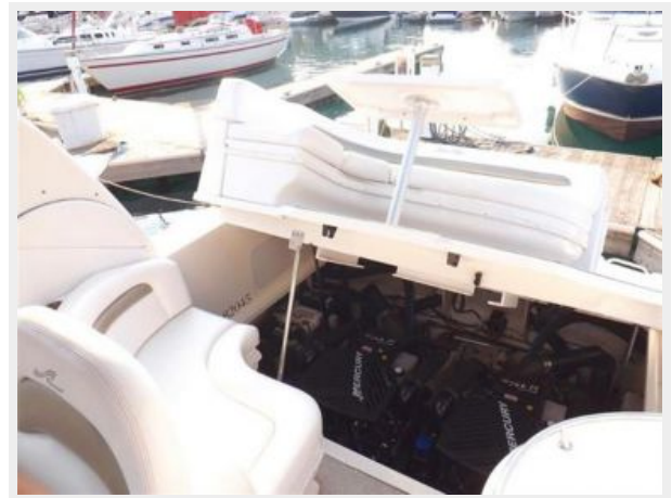
Hydraulic engine room hatch
