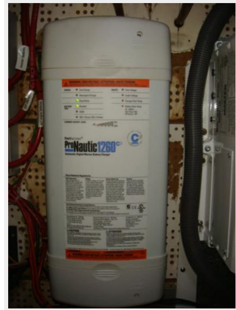
48' Defever Battery Charger
