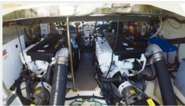
Volvo Penta IPS engine room
