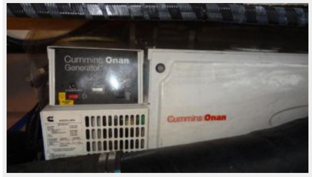
New Onan 9kw Generator w/ Sound Shield
