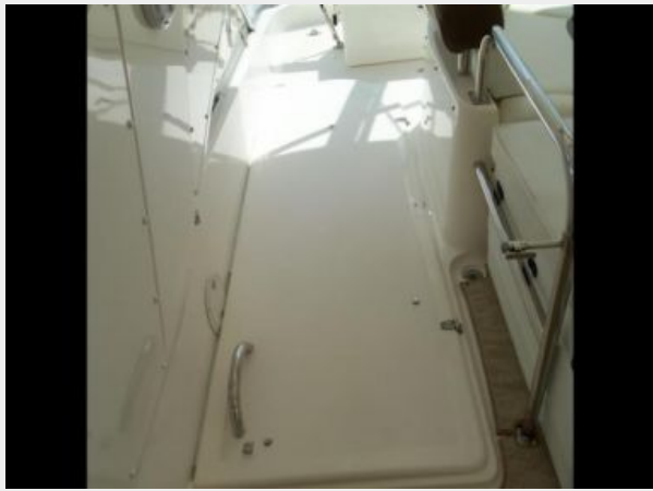
Hinged Door Over Flybridge Stairs
