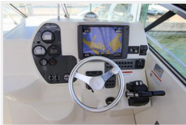
Helm Station W/Digital Engine Gauges & Touchscreen Garmin
