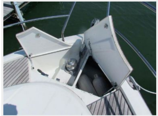
ANCHOR WELL & WINDLASS
