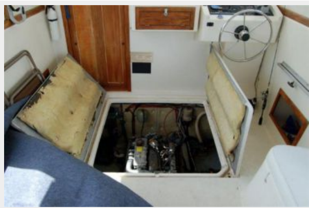
Engine Access Hatch
