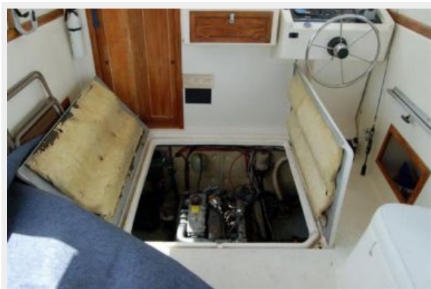
Engine Access Hatch
