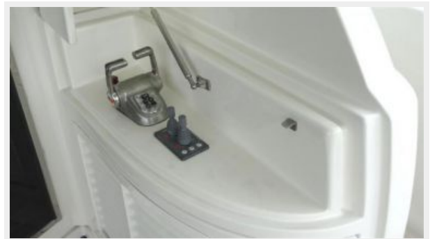
Aft Deck Controls with Thrusters
