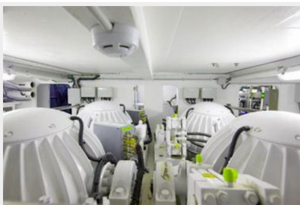
Seakeeper zero-speed stabilization
